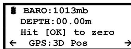
If the depth is not reading zero (this is possible if the probe is wet and a low EC reading is registering), press the OK key. You will be asked to confirm by pressing OK again.
