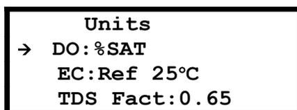
On this screen you can adjust the DO: setting between %Sat and mg/L. This will set the Dissolved Oxygen output to AquaLink to as either % Saturation or in milligrams/Litre (which is the same as parts per million). Both readings are automatically corrected for atmospheric pressure, sample temperature and sample salinity.
