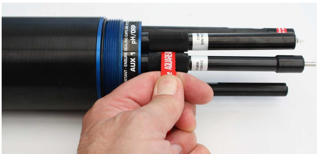
Slide the lanyard over the electrode and use it to grip the knurled body.
