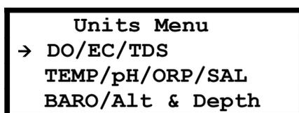
At the Units Menu, you have a choice of which units you want to adjust. Choose the first line if you want to adjust Dissolved Oxygen, Electrical Conductivity or TDS. Choose line 2 if you want to adjust Temperature, pH, ORP or Salinity. Finally, line 3 will give access to Barometric Pressure, Altitude and Depth settings.
