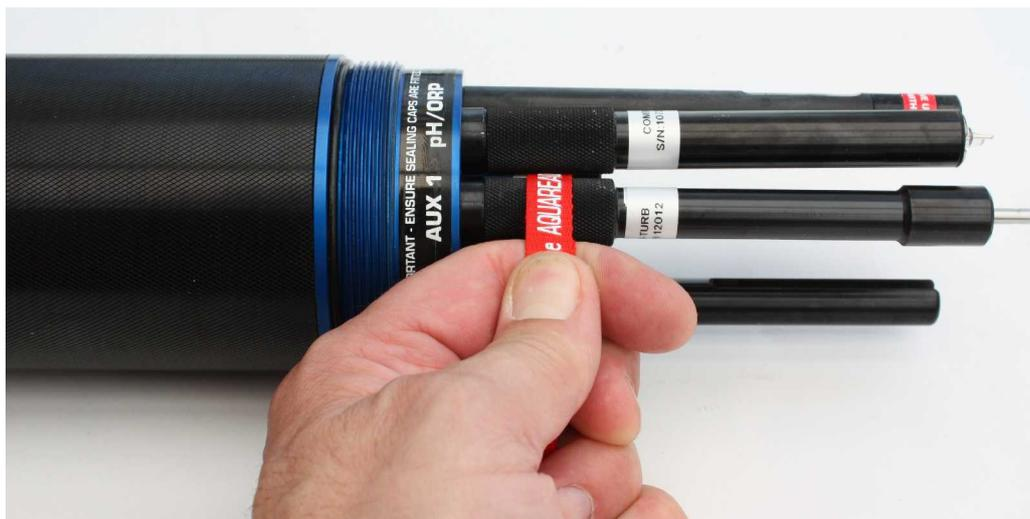
Apply a small amount of silicone grease (supplied with the AP-5000) to the threaded section and the O-ring of the AUX Electrode (see photograph).
