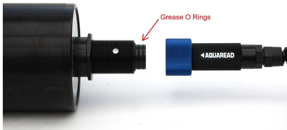
Apply a generous smear of grease to the O-rings where indicated above. Be careful not to get any grease inside the connector near the gold contacts. A small smear of grease should also be applied to the thread on the Probe to allow easy tightening of the collar.
