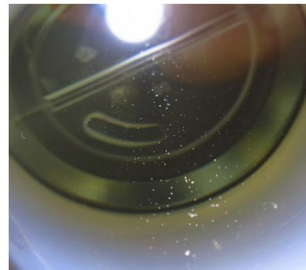
The photograph to the right was taken in a calibration bottle after fresh water was poured in. The bubbles are clearly visible in the light beam. This level of aeration will register the equivalent of around 5NTU as each bubble is seen as a solid particle.
