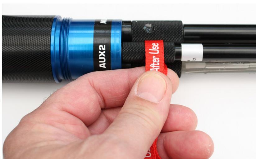
Apply a small amount of silicone grease (supplied with the Aquaprobe®) to the threaded section and the O-ring of the AUX Electrode (see photograph). **ENSURE NO GREASE IS APPLIED TO THE GOLD CONTACTS.**
