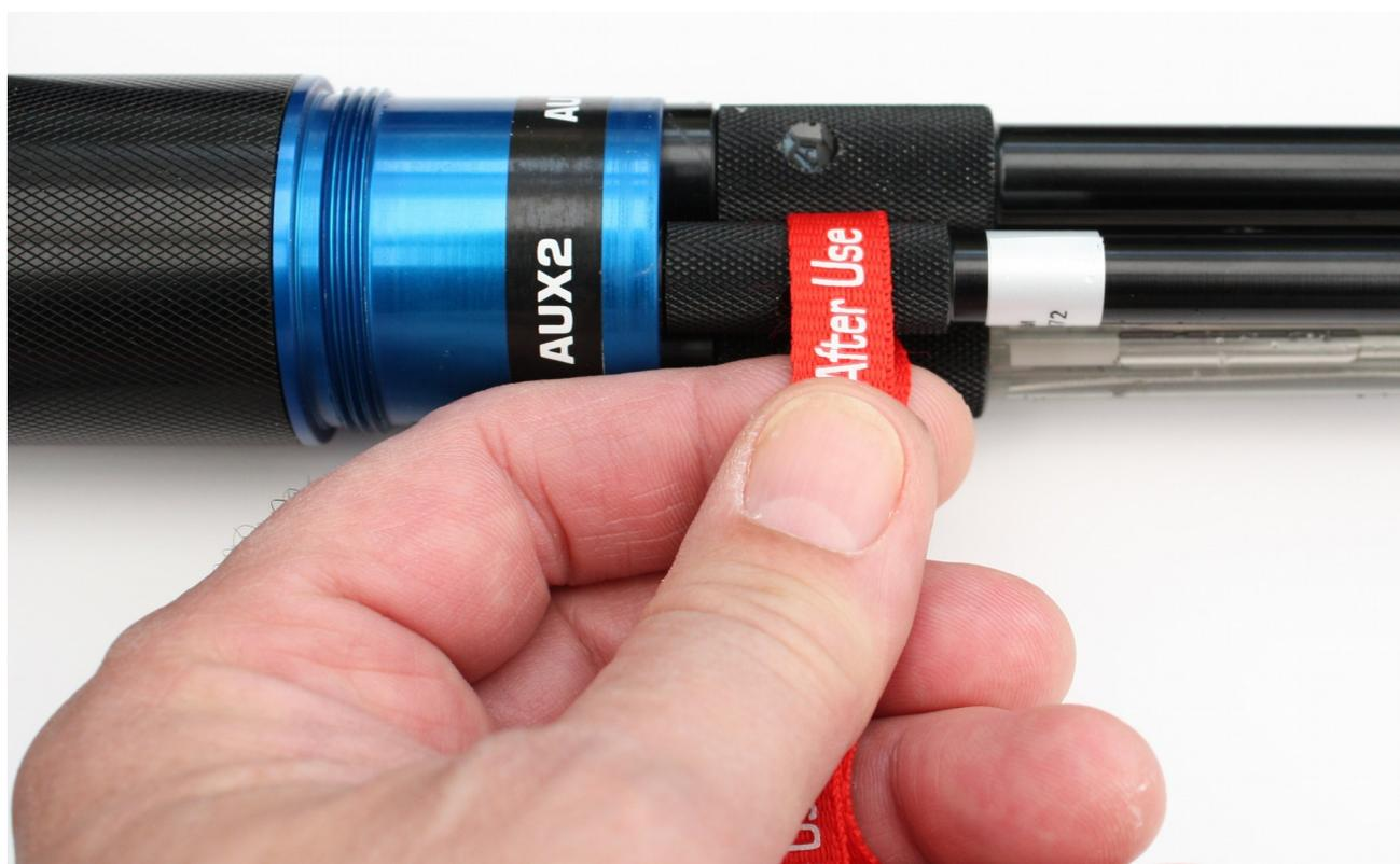
Slide the lanyard over the electrode and use it to grip the knurled body.
