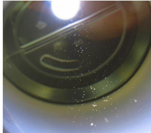
If a zero point calibration is conducted under these conditions, when the Probe is subsequently deployed in clear water it will register a negative reading between -5 and -10 NTU.
