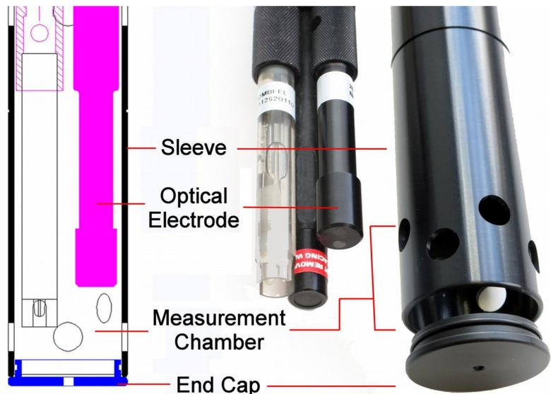
**In order to obtain consistent results, the measurement chamber created within the Aquaprobe® must remain physically constant during both calibration and measurement.**
