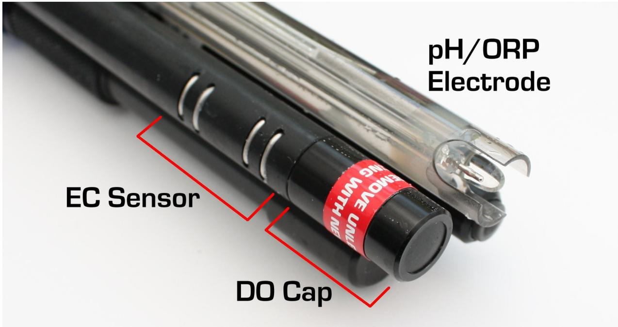
Please note: The photograph shows the AP-2000 with Optical DO. The AP-700 and AP-800 models may have either Optical DO or Galvanic DO sensors.
