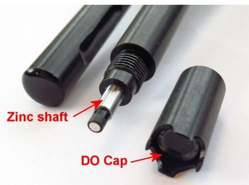
**NEVER re-install a Galvanic DO Membrane Cap once it has been fully tightened.** The membrane will be stretched and will not seal properly over the silver cathode a second time. If the membrane does not create a proper seal over the silver cathode, the DO sensor will not operate correctly and any readings given will be erroneous.
